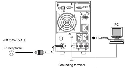
Connect the ground wire to the Grounding terminal.
